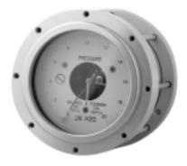
For test laboratory and production uses, this gauge gives accuracy and is compact in size. It is sensitive, yet rugged and low in cost. Available in 18 standard ranges (including vacuum and compound ranges), the Series 300 is convenient to use. High differential pressure is applied to the capsule; low pressure to the case. Maximum static (case) pressure is 150 psig.
